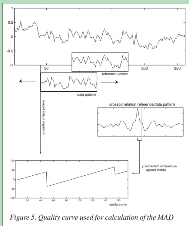
Figure 5. Quality curve used for calculation of the MAD
